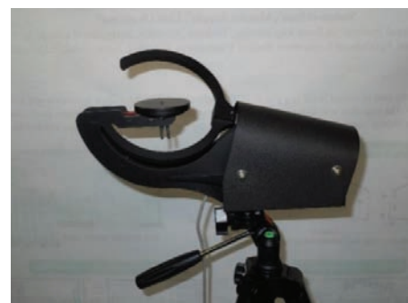
Figure 10 Global and diffused radiation sensor
